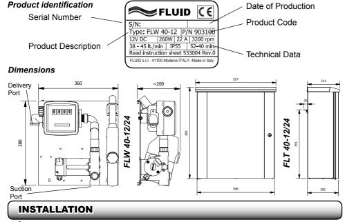
**DANGER!** If the application is for gasoline, petrol or fluids that require an explosion-proof product, DO NOT INSTALL THIS ELECTRIC PUMP.
